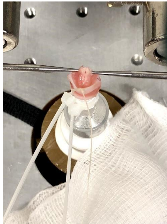
Figure 6. Single pronged micropositioners. These were used to adduct rabbit arytenoid cartilages and bring the vocal folds closer together. Cable ties were used to secure the trachea to the pseudolung.
