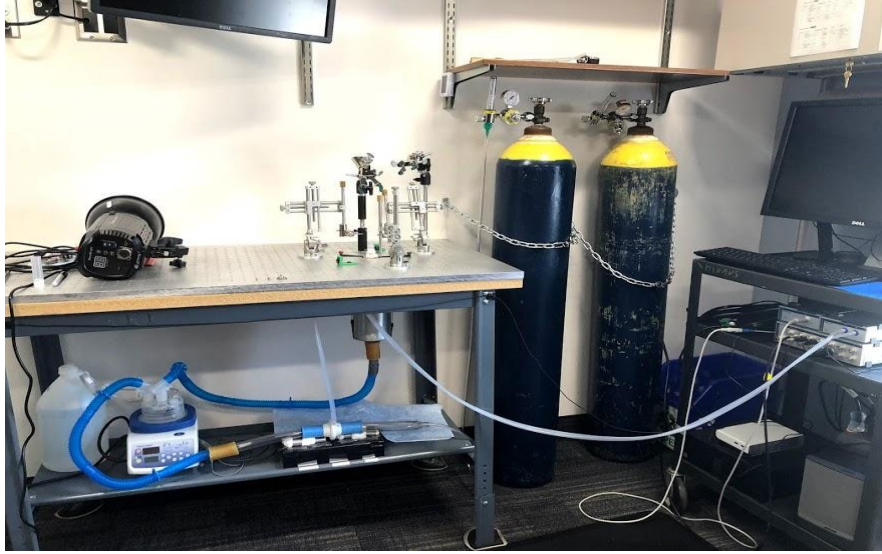
Figure 2. The benchtop apparatus. Included in this picture are the humidifier, the signal acquisition system, the computer and monitor, the pseudolung, and the air tanks.
