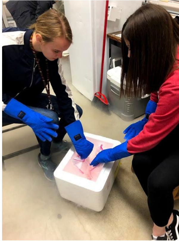
Figure 1. The flash freezing process. Pig larynges were submerged in PBS solution in either gallon plastic bags or plastic cylindrical containers and placed in liquid nitrogen. Rabbit larynges were also flash frozen according to protocols at the University of Utah.
